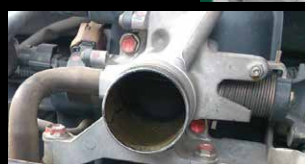
BEFORE (Throttle body condition after 60,000 km)
